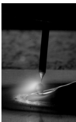
Droplet detachment after the pulse phase
