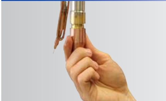
Step 1: Screw off the gas nozzle
