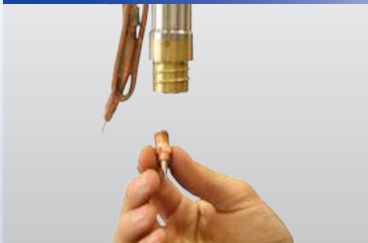
Step 3: Insert a new electrode
