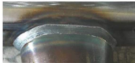
Mild steel / intersecting wire welding Thickness 1.5mm, Current 95A, Voltage 17V Welding speed 50cm/min Gas (80% Ar + 20% CO 2 )
