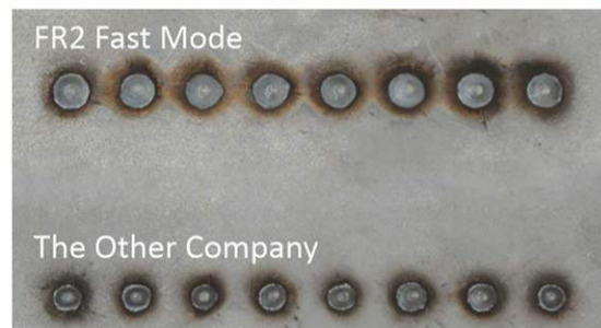
Mild steel / spot welding Thickness 3mm, current 160A Unified voltage Spot welding time: 0.6 seconds
