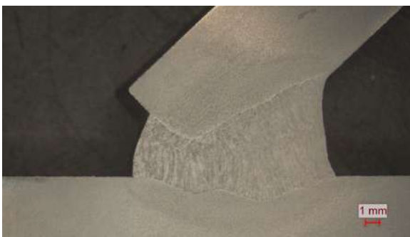
Material thickness: 10 mm, included angle: 35°
