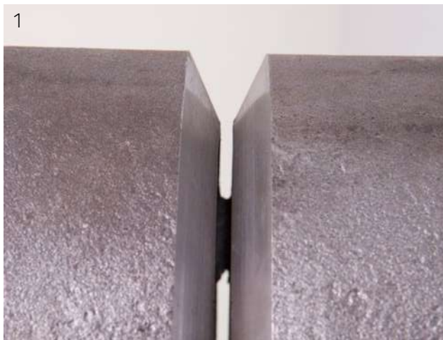
1 Weld preparation of root welds on pipes, 60° included angle with 3 mm air gap
