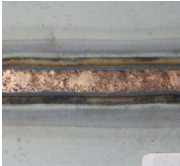
Brazing galvanized sheet metal
