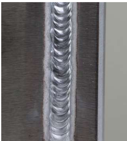
AlMg5, material thickness: 4 mm
