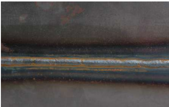
Root welding in PC position with an air gap and without weld pool backing
