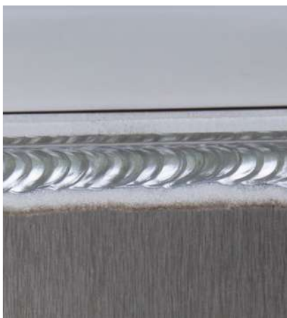
AlMg5, material thickness: 4 mm
