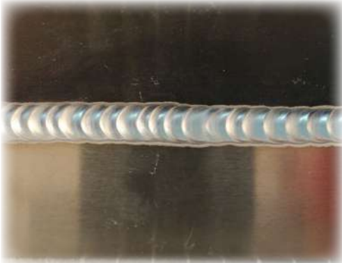
Visible TIG seam: uniform bead ripples even on long seams
