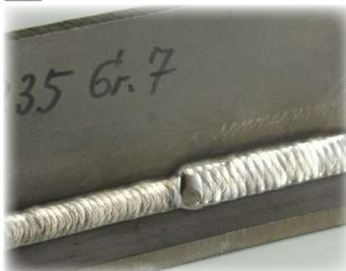
PB Filler and final pass, titanium grade 7 (3.7235)
