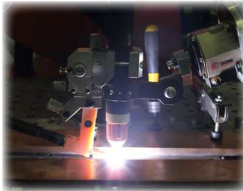
PA Fully mechanised welding process
